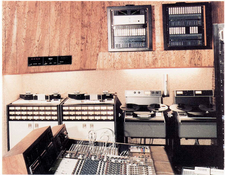
Audio Tonstudios of Berlin offers the versatility of a 46-channel automated mix using synchronized MM-1200s and ATR-100s.
